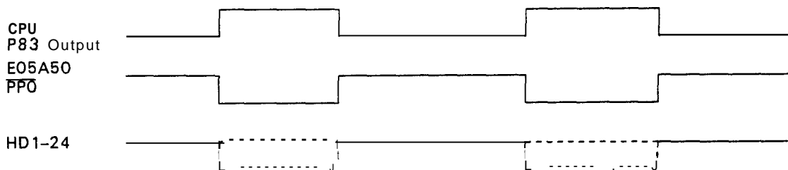
Figure 2-25. Head Drive Signal Output Timing
