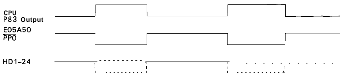
Figure 2-25. Head Drive Signal Output Timing
